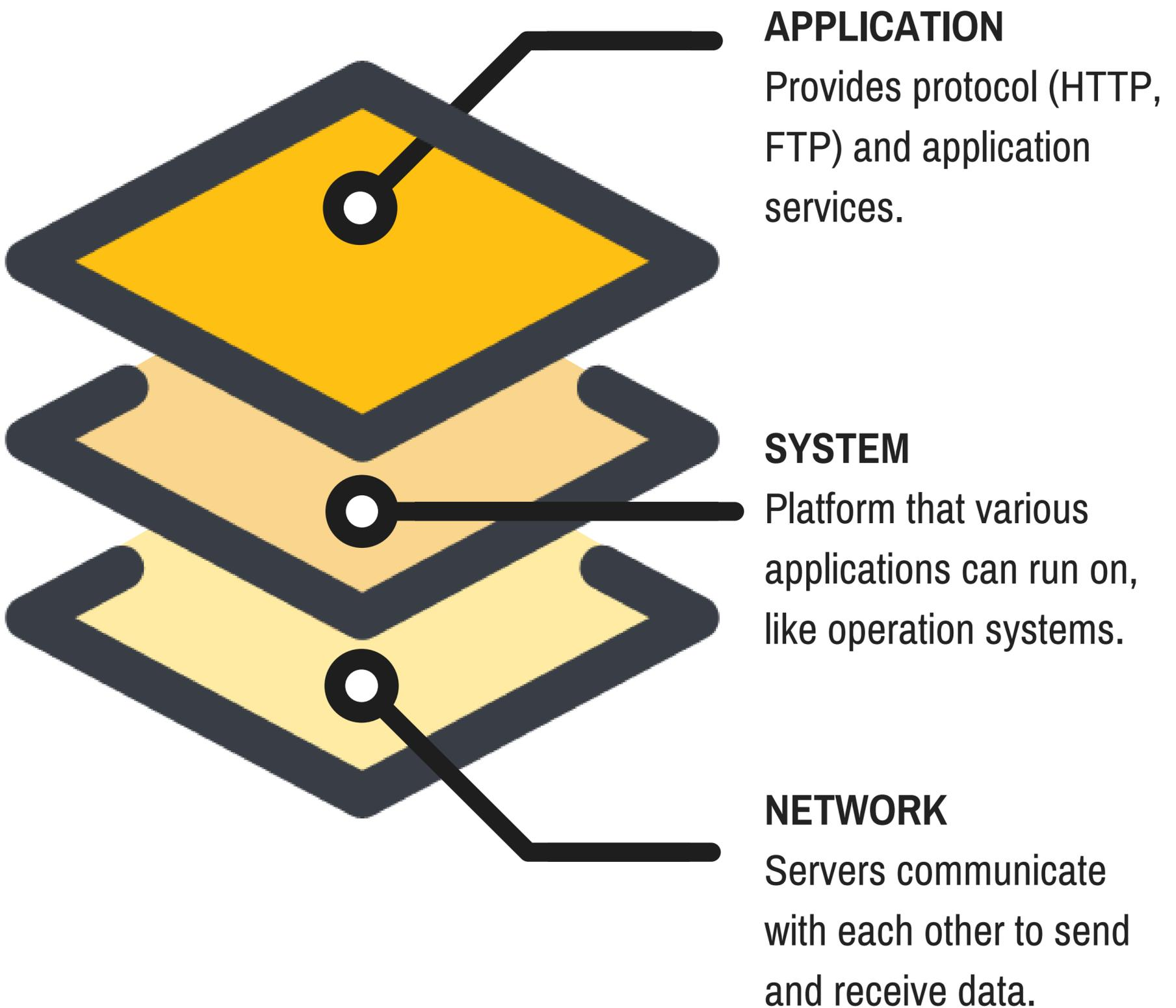
An IT system, therefore, consists of a **network** layer, a **system** layer, and an **application** layer. These three layers interact with one another to make IT systems work.\*
